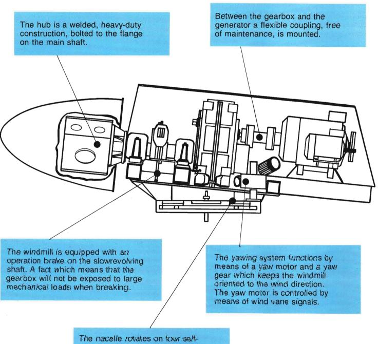
The nacelle rotates on four selfgreasing Oilon blocks, mounted between the cabin and the year gear wheel.
