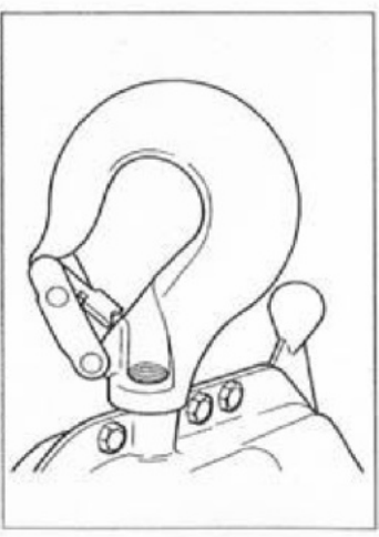
Fig. 10a - Correct slinging.
