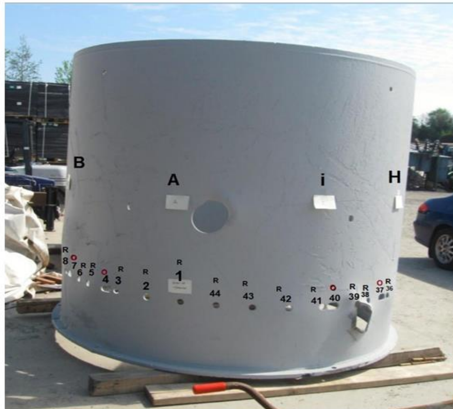
Foundation Can - Numbered Re-bar Holes for Illustration
