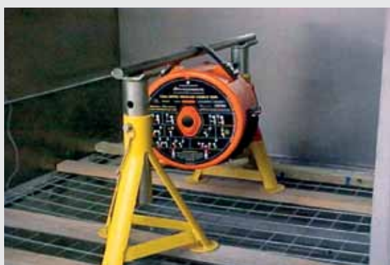
ManSafe® Sealed SRL before and after dust test.
