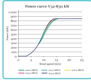
The figure above illustrates the power curves at different sound levels for the V52-850-kW turbine, which is equipped with OptiSpeed®.
